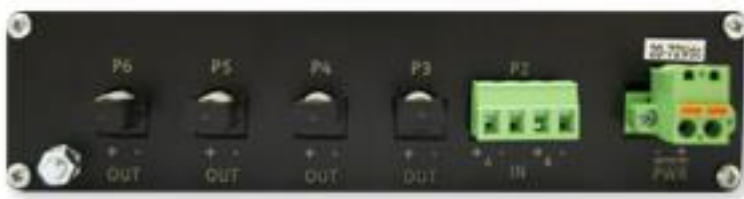
Figure 3 – Rear panel of ITD, configured with four fiber outputs
