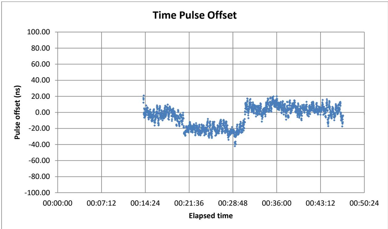
Figure 1: Pulse offset of TTM 01-G from reference over time
