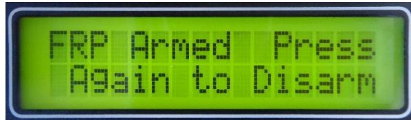
Figure 3 - Message indicating that Factory Reset is armed
