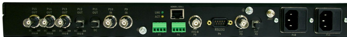
Figure 12 – Rear panel of TCG 02-G, with IEC-320 power connectors and BNC and Fiber outputs (P2 and P3)
