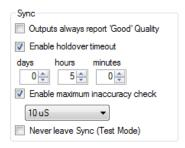
• Improvement: Added the ability to suppress individual IRIG-B or Programmable Pulse outputs based on inaccuracy threshold or holdover timeout. The feature is available in firmware 3.21r3 (NTS 02-E, NTS 03-E, NTS 02-G, NTS 03-G) and TCG E series firmware 2.25r5. When "holdover timeout expires" is selected, that particular output will stop providing a time signal when the clock is out of sync and the specified holdover time has expired.
